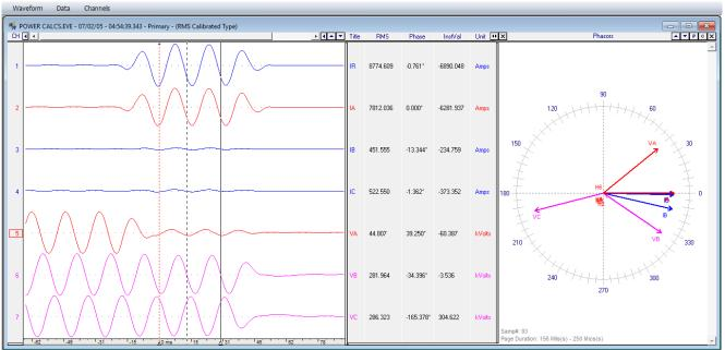
**<u>Step 1:</u>** Select a current and voltage waveform and press enter to isolate the two.
